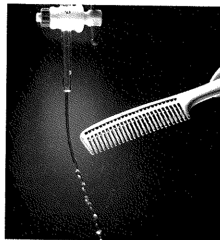
Figure 3.11 In this photo, the comb is charged, and the water is neutral.
