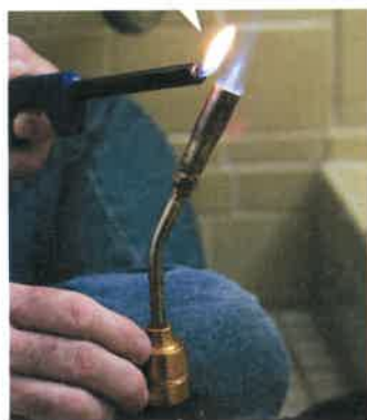
Figure 2.17 A lighter provides energy to start the reaction between oxygen and propane. Predicting: If energy input was not needed to light this torch, what would happen when propane was released from the tank?
