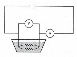
b. If the voltmeter reading holds steady at 50.0 V and the ammeter reading holds steady at 5.0 A, estimate the time in seconds required to completely vaporize the water in the beaker. Use 4200 J/kg·C° as the specific heat of water and 2.30 × 10<sup>6</sup> J/kg as the heat of vaporization of water.
