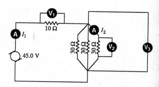
The three resistors in parallel have a total resistance of
