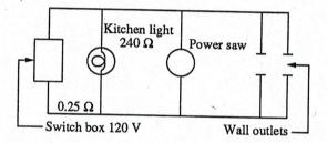
a. Compute the effective resistance of the circuit consisting of just the light and the lead lines to and from the light.
