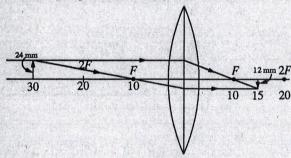
14. An object 2.25 mm high is 8.5 cm to the left of a convex lens of 5.5-cm focal length. Find the image distance and height.
