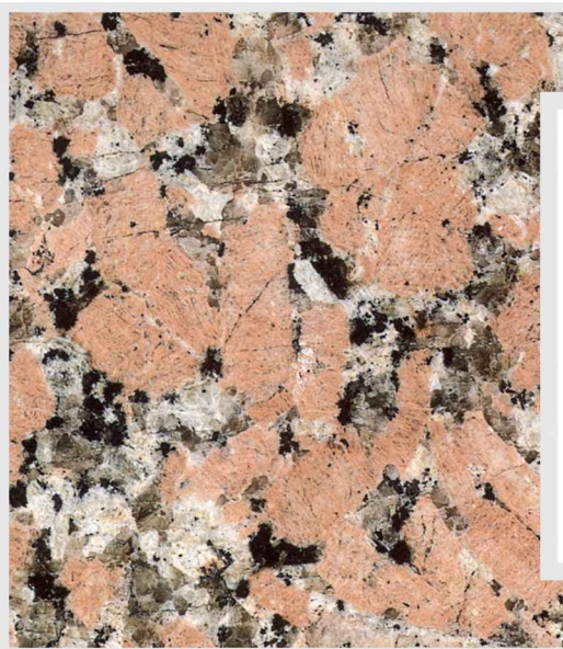
A close-up image of a polished piece of granite, an igneous (plutonic) rock with many similar-sized crystals of orthoclase (pink), biotite (black), albite (white), and quartz (gray); see Chapter 7.
